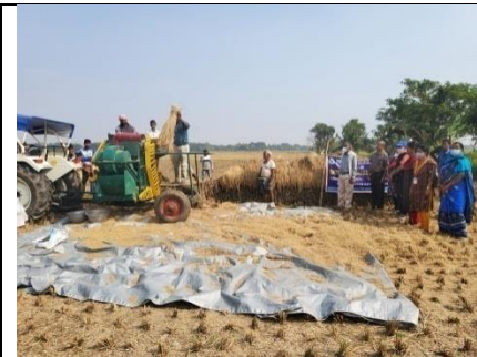
Demonstration of Tractor drawn Whole straw Thresher to produce bundle straw for mushroom production
