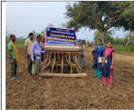
Demonstration of tractor drawn Zero till Seed cum Fertilizer drill for line sowing of Greengram
