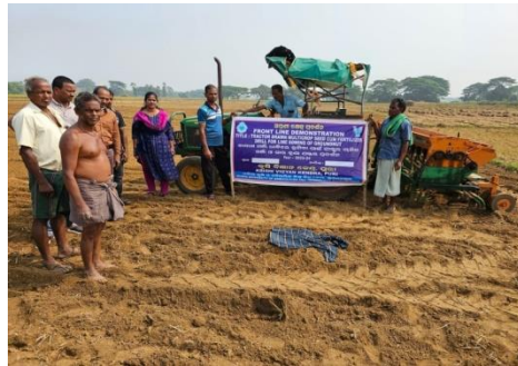
Demonstration of tractor drawn 9-row multi crop seed cum fertilizer drill for sowing of groundnut
