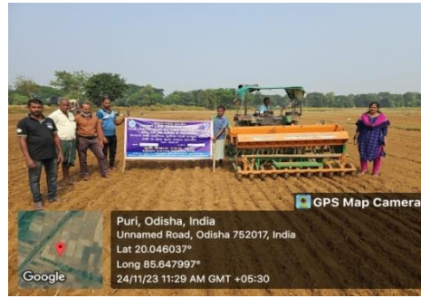
Demonstration of tractor drawn 9-row multi crop seed cum fertilizer drill for sowing of groundnut
