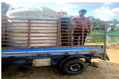
Transportation of live fish yearlings by using a water storage tank & O 2 cylinder
